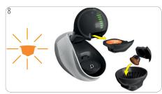
Used capsule icon blinks orange until capsule is removed. Pull out capsule holder. Remove used capsule. Put used capsule in capsule bin.
