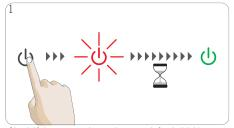
Check if the water tank contains enough fresh drinking water. Switch on machine. While machine is heating up, ON / OFF icon starts blinking red. After approx. 30 seconds, ON / OFF icon lights up steady green. Machine is ready to use.
