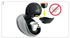
Pull out capsule holder. Make sure rinsing tool is not inside. Insert capsule in capsule holder. Insert capsule holder into machine.
